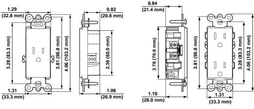
**DUPLEX BACK AND SIDE WIRED,** SINGLE BACK AND SIDE WIRED, SELF-GROUNDING SELF-GROUNDING Sold by Cat. No. 16252 Cat. No. 16251 TWAcomm●com http://www.TWAcomm.com Toll Free: (877) 892-2666
