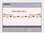
Troubleshooting starts here. See a diagram of the channel, including patch cords. Check that the link is patched all the way across the campus, and identify how many connectors are in a link.
